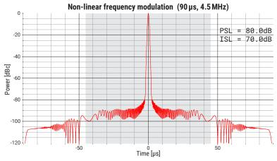
PSL = Peak Sidelobe Level: distance between correlation peak and first range sidelobe in dB ISL = Integrated Sidelobe Level: difference of peak power and integral of all range sidelobes in dB
